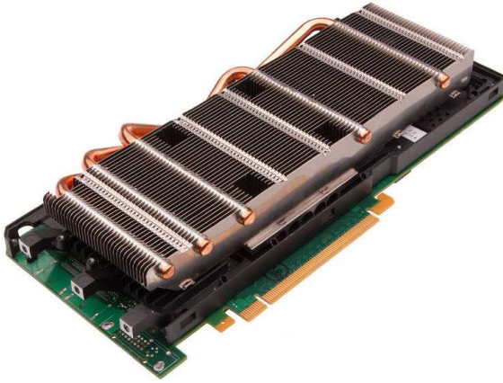
Figure 1: The Nvidia Tesla M2090 GPU, capable of 665GFLOPs of double-precision floating-point arithmetic in a power envelope of 250W. It is designed to be attached to a 16-line PCI Express version 2.0 interface within a high-performance compute cluster node.
